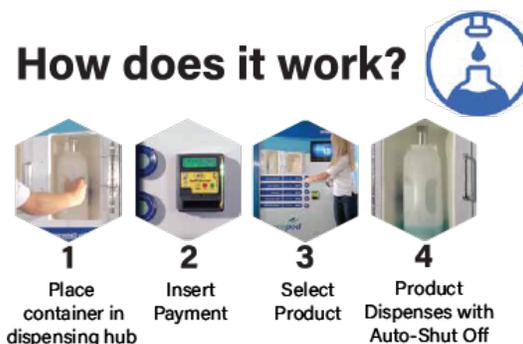
The Ecopod system dispenses up to five products, which are stored in 15-gallon canisters in the back of the module. For larger volume products, 30-gallon canisters are also available. When a canister is running low on a product, the system sends a message to a designated iPhone. The empty canisters can be easily replaced with a full canister by existing employees. Empty canisters are then collected for refilling and redistribution.
